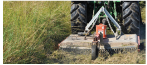
Decontaminate recesses and crevices on slashers
