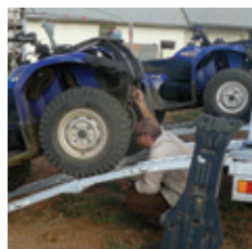
Remove belly plates for inspection
