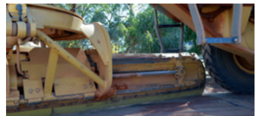
Decontaminate front and back of grader blades and hydraulic rods
